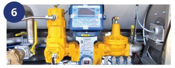
Combination of Liquid Controls mechanical flow meter MA-7 with S.A.M.P.I. electronic head, used mainly in Poland, Romania and Bulgaria.
