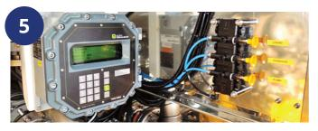
Combination of Liquid Controls mechanical flow meter MA-7 with Horn Tecalemit electronic head.
