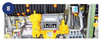
Liquid Controls mechanical flow meter MA-7-GX-10, the most frequent flow metering solution on road tankers, currently on the decline. Most often used in all LPG markets.
