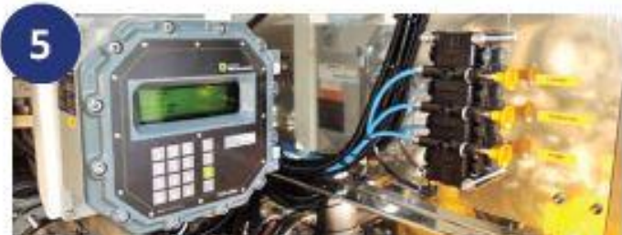
5 Combination of Liquid Controls mechanical flow meter MA-7 with Horn Tecalemit electronic head.
