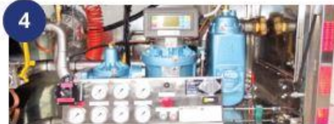
4 Mechanical flow meter with PERNIN electronic head, popular in France.
