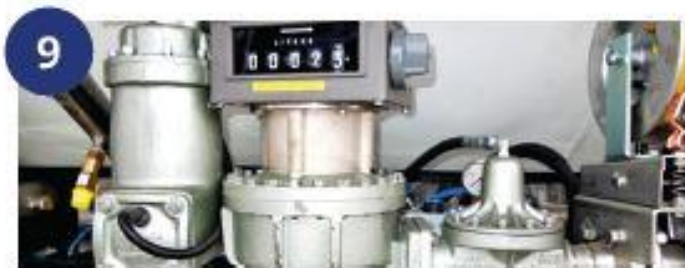
9 Liqua Tech mechanical flow meter LPM-200 – supplied mainly to Russia and Ukraine. Not MID certified.
