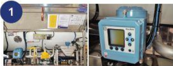
1 VPS/MS/LPG mass flow metering system – the most modern system assembled from EMERSON brand components. The most frequently used system in CZ, PL, SK, D, RU, BY, LT, LV, EST and UA markets.
