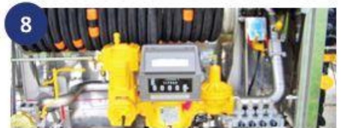
8 Liquid Controls mechanical flow meter MA-7-GX-10, the most frequent flow metering solution on road tankers, currently on the decline. Most often used in all LPG markets.
